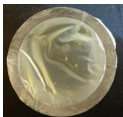
Fig.1. A top view of the feeding chamber used to screen the bacteria through the aphids. Parafilm (a stretchy plastic-similar to cling film) is stretched over a plastic cylinder to form a film over the top. The artificial diet is put on to this film. Another layer of Parafilm is then stretched on top to create a sachet. Aphids are then put inside the cylinder. The aphids move up to the food source and feed as they would from a leaf.
